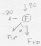
$$F_{CF} \cdot \sin 45^\circ = 20 \\ F_{CF} = 28,28 \text{ kN} \\ 20 + F_{FD} + F_{CF} \cdot \cos 45^\circ = 0 \\ F_{FD} = -40 \text{ kN}$$
